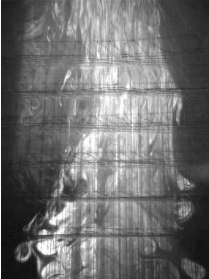
FIGURE 4. LIF visualization for 155 \leq z/d \leq 255 ( Re = 2000 , G = 9.2 ). The flow is from bottom to top. Bright horizontal lines in the viewframe indicate location of the grids, while dark vertical lines are shadows from the wires.
