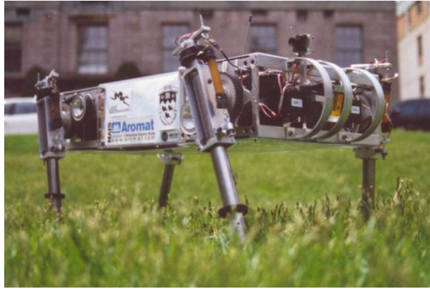
Fig. 1. Scout II: A high performance, power autonomous, four-legged robot with one actuator per leg.
