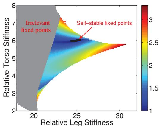
**Figure 3:** Fixed points computed for the same total energy, average speed and hopping height and for different values of dimensionless leg and torso stiffness. The color code corresponds to the values of the spectral radius of  $A$ .
