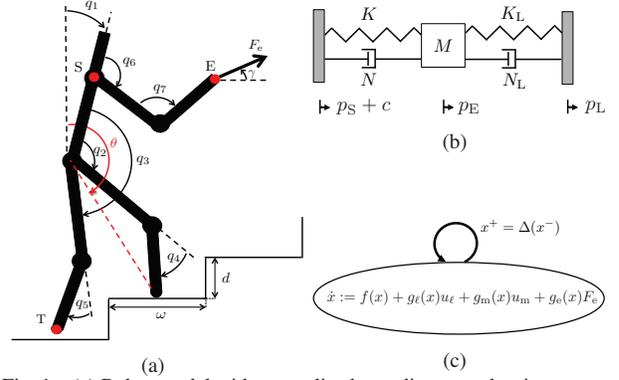
Fig. 1. (a) Robot model with generalized coordinates and stair geometry (b) Impedance model of interaction task (only horizontal component is shown). (c) Overall hybrid dynamics of the biped.
