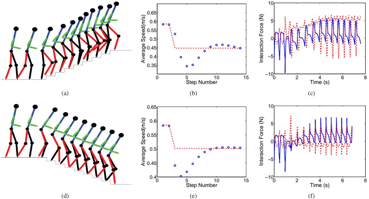
Fig. 3. **Top:** Simulation results when transitioning from flat ground to upstairs. **Bottom:** Transitioning from flat ground to downstairs. (a) and (d) Snapshots of walking. Black and red links correspond to the stance and swing foot respectively. (b) and (e) Average walking speed of the biped (blue markers) and desired speed of leader (red line). (c) and (f) Interaction force. Solid blue is the horizontal component and dashed red is the vertical component.
