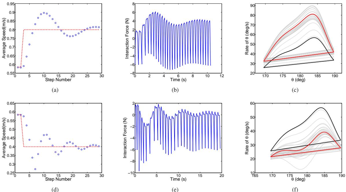
Fig. 2. **Top:** Biped response when the leader increases speed. **Bottom:** Biped response when the leader decreases speed. (a) and (d) Average speed of the leader (dashed red line) and average speed of the biped (blue marker). (b) and (e) Horizontal component of the interaction force. (c) and (f) Convergence of limit cycles. Black is the base (unforced) limit cycle, gray is the transitioning and red is the final limit cycle.
