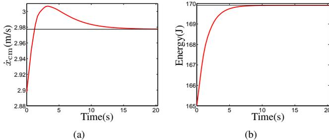
Fig. 7. Evolution of the horizontal velocity (a) and total energy (b) at anterior touchdown in response to a  $0.08\text{m/s}$  disturbance in  $\dot{x}_{cm}$ ; black lines correspond to nominal values.
