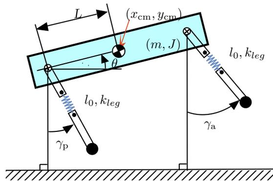
Fig. 1. A sagittal-plane bounding model with massless legs.
