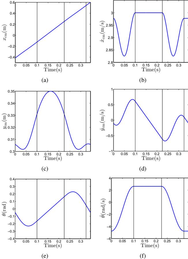
Fig. 3. State evolution at a symmetric bounding gait starting at anterior leg touchdown. Vertical lines represent subsequent events; from left to right: anterior leg liftoff, posterior leg touchdown, posterior leg liftoff.
