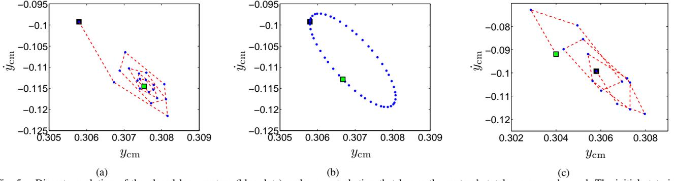
Fig. 5. Discrete evolution of the closed loop system (blue dots) under a perturbation that leaves the system’s total energy unchanged. The initial state is marked by the black square while the final condition is marked as green square. 5(a):  $c = 0.5$ ; 5(b):  $c = 1$ ; and 5(c):  $c = 1.2$ .
