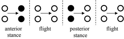
Fig. 2. Footfall pattern of a nominal bounding gait; solid circles indicate legs in contact with the ground and white circles indicate legs in the air.
