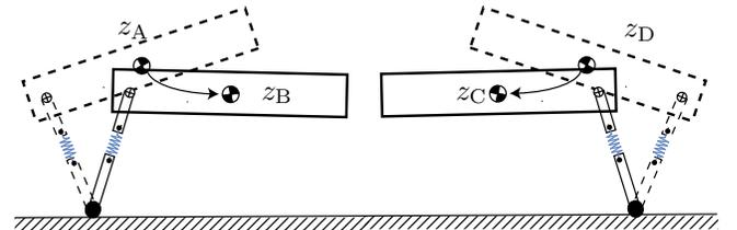
Fig. 4. The stance-posterior and stance-anterior phases are related through a time-reversal symmetry.
