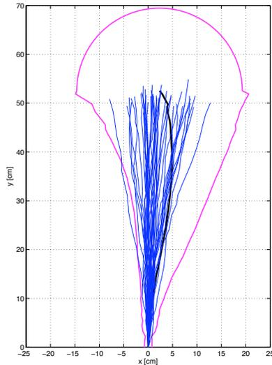
Fig. 6. Output of the stochastic model, tuned using Monte Carlo simulation. The 45 model instantiations, shown in blue, correspond to the values  $\sigma_i^{\max}$  of Table III and are plotted over the average (in thick black) of the whole data collection. The 95% confidence level still allows a few paths to go outside the marked (in magenta) confidence region.
