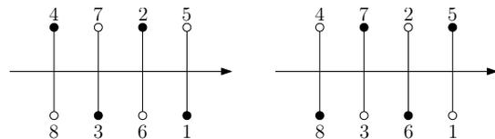
Fig. 2. Foot fall pattern of the OctoRoACH robot
