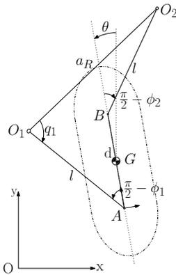
Fig. 4. Analysis of the mechanism.  $d$  is the distance between the hip points and  $l$  the leg length. The angle  $\theta$  is used to denote the orientation of the model with respect to some global frame of reference.
