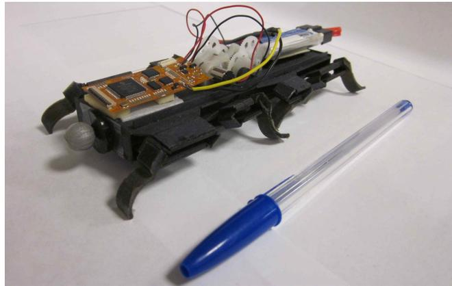
Fig. 1. The OctoRoACH robot, designed by A. O. Pullin [9] at the University of California, Berkeley and manufactured by Motile Robotics, Inc. The robot has a total mass of 35 gm, its body size is 130x60x30 mm and the maximum speed it can reach is 0.5 m/s.
