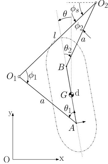
Fig. 6. Kinematic analysis of the four-bar mechanism that describes the problem.  $a, d$  are parameters that define the size of the mechanism,  $O_1, O_2$  and  $\phi_s$ , after being defined, remain fixed for the rest of the sweeping phase.
