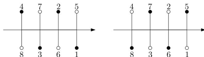
Fig. 3. The foot fall pattern of the robot which is a tetrapod gait.
