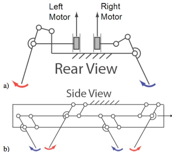
Fig. 2. Leg kinematics: a) The slider-crank linkage, responsible for the abduction and adduction motion (in and out motions from the sagittal plane) of the legs and b) the parallel four-bar mechanism which enables protraction and retraction of the legs. (Courtesy of A. O. Poullin; reproduced from [9] with the author’s permission.)
