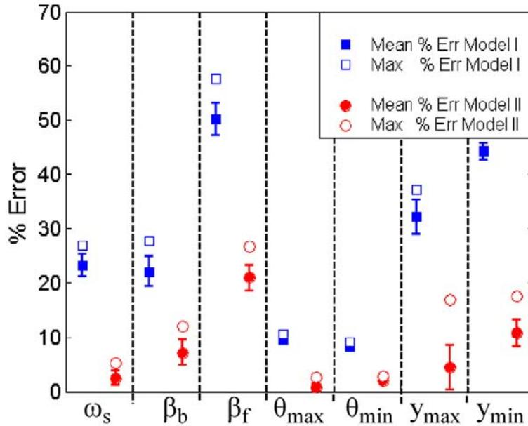
**Figure 16. Mean and max errors between simulation models and experimental results in gait parameters and max and min values of the pitch and hopping height over 70 bounding strides at average forward speed approximately 1.3 m/s.**
