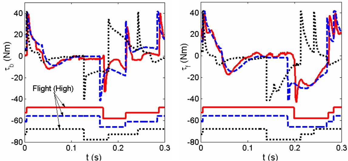
**Figure 14. Back (left) and front (right) torques. Experimental data (solid), Model I (dotted) and Model II (dashed) during one step. The square wave represents the leg states: Flight (high), stance-retraction (low) and stance-brake (medium).**
