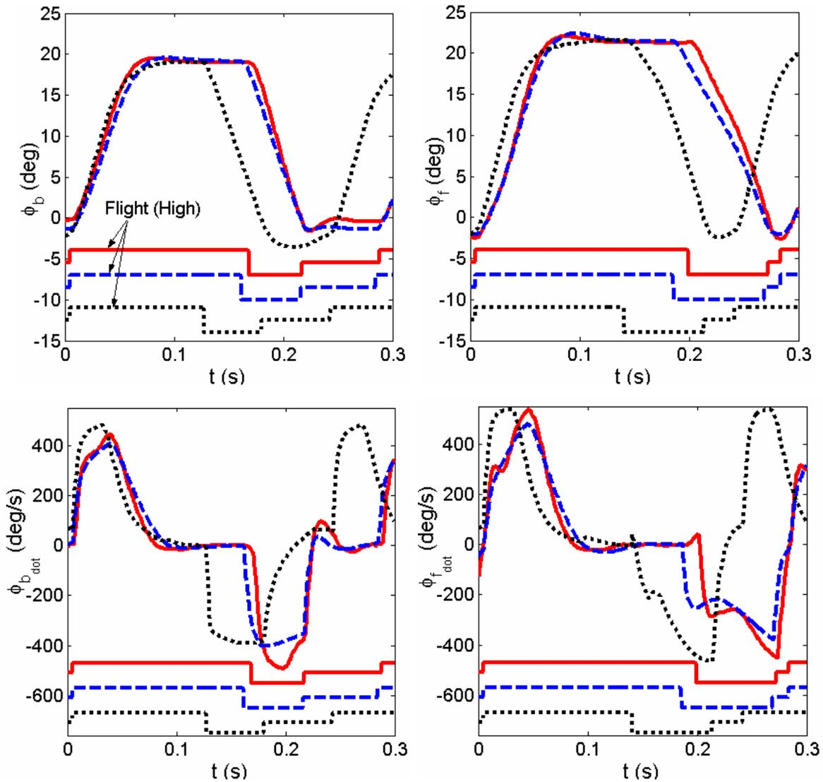
**Figure 13. Back (left) and front (right) leg angles (upper) and leg angular velocities (lower) during one step. Experimental data (solid), Model I (dotted) and Model II (dashed) during one step. The square wave represents the leg states: Flight (high), stance-retraction (low) and stance-brake (medium).**
