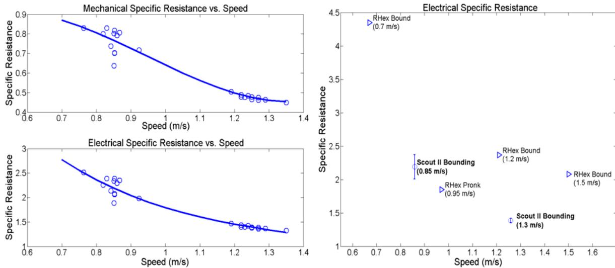
**Figure 7. Specific resistance for Scout II based on mechanical and electrical power (left) and specific resistance based on electrical power for Scout II and RHex [7]. Error bars indicate standard deviation.**
