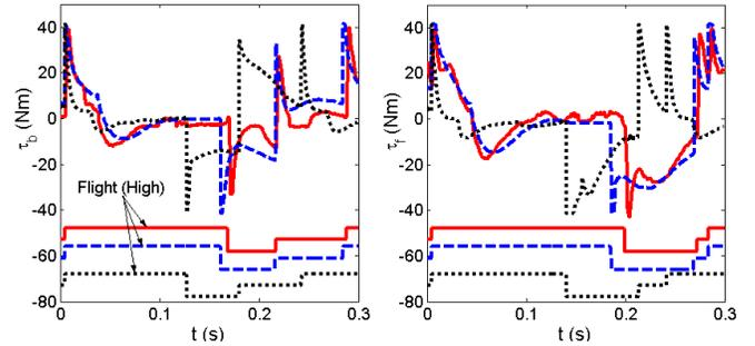
Figure 10. Back (left) and front (right) leg torques during one step. Experimental data (solid), Model I (dotted) and Model II (dashed). The square wave represents the leg states: Flight (high), stance-retraction (low) and stance-brake (medium).
