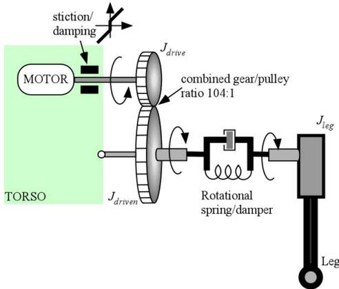
Figure 6. Details of the hip unit model.
