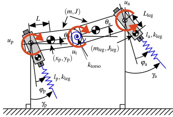
**Fig. 1** The sagittal-plane quadrupedal model with a flexible torso and non-trivial leg mass.
