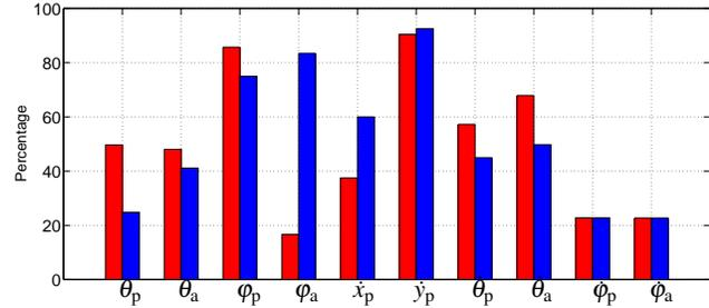
**Fig. 6** Ratio of the largest single perturbation that can be tolerated as predicted by the SOS method over the corresponding value obtained by numerical simulation. The red and blue bars correspond to the positive and negative perturbations, respectively.
