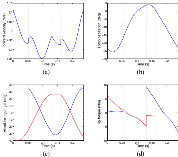
**Fig. 3** Evolution of forward velocity (a), torso oscillation (b), absolute leg angles (c) and hip joint torque (d) of a fixed point. In (c) and (d), the red and blue lines correspond to the anterior and posterior legs, respectively. The vertical lines separate one cycle into four phases: from left to right, fg, sp, fe and sa. The discontinuities are due to the impact at touchdown.
