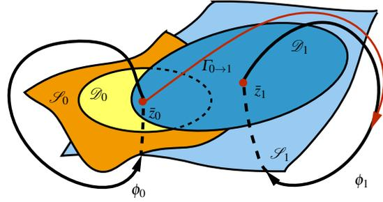
**Fig. 5** A conceptual illustration of the transition between two limit cycles, i.e.,  $\phi_0$  and  $\phi_1$ .  $\mathcal{S}_0$  and  $\mathcal{S}_1$  are the Poincaré sections of  $\phi_0$  and  $\phi_1$ , and  $\bar{z}_0$  and  $\bar{z}_1$  are the corresponding fixed points.  $\mathcal{D}_0$  and  $\mathcal{D}_1$  are the domain of attractions at the Poincaré sections for  $\phi_0$  and  $\phi_1$  respectively.
