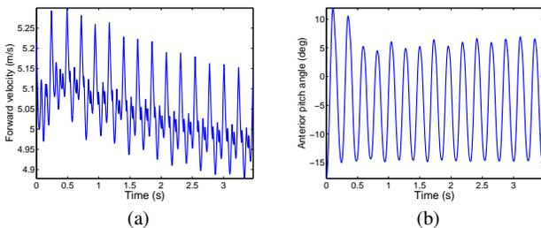
**Fig. 4** The evolution of the forward velocity and the anterior pitch when the system is perturbed with  $+0.1\text{m/s}$  in  $\dot{x}_p$  and  $-3\text{deg}$  in  $\theta_a$ .
