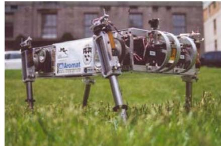
Figure 1. Scout II: A simple four-legged robot.
