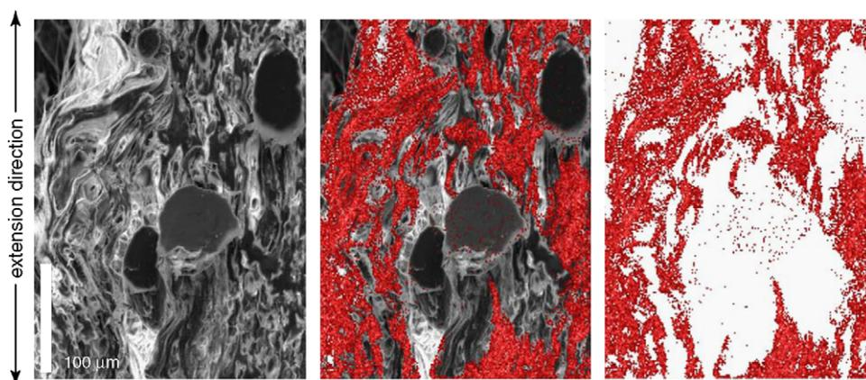
Fig. 13. Energy dispersive spectroscopic fluorine dot mapping of the expanded specimen after extension and removal from the test fixture. From left to right: SEM image of the mapped area; the fluorine dot map overlaying the image; the fluorine dot map. The PTFE is clearly identifiable as the fibrillating phase.
