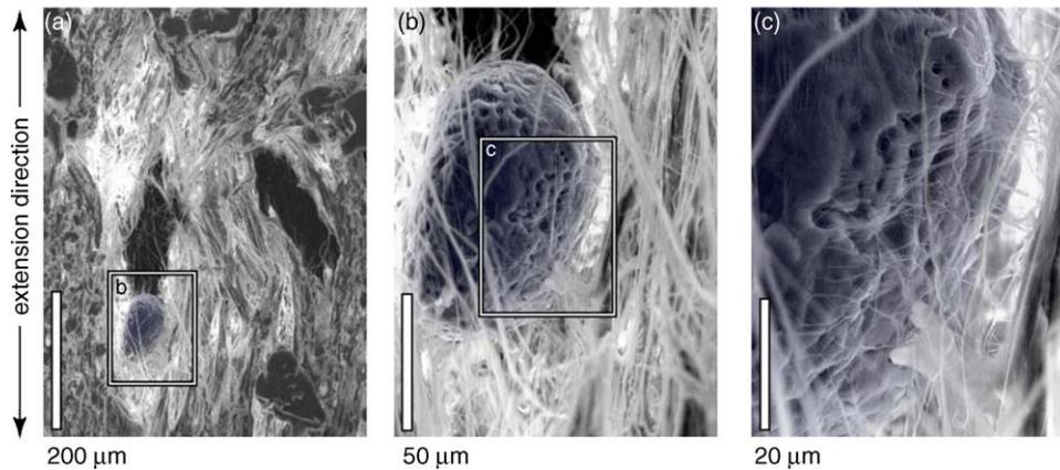
Fig. 14. Scanning electron images of the 30 wt.% fracture sample. This sample was extended, removed from the test fixture and carbon coated. From left to right: low magnification image revealing an undamaged PEEK particle; increased magnification image of the particle showing highly fibrillated microscale PTFE encapsulating the particle; high magnification image showing a networked structure of nanoscale PTFE fibrils trapped within the coalesced PEEK particle.
