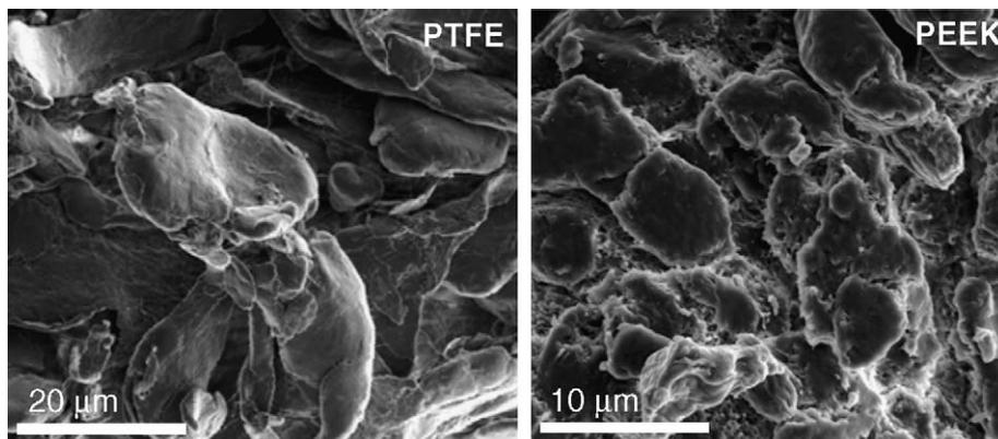
Fig. 2. Scanning electron micrographs of the constituent powders before jet-milling. Both materials are agglomerated prior to blending, and the blend material is compression molded to make this PTFE-PEEK composite. The PTFE and PEEK agglomerations have characteristic sizes ranging from 100 to 1000 and 10–40 μm, respectively. The disbanded PTFE and PEEK particles have characteristic sizes ranging from 5 to 25 and 2–10 μm, respectively.
