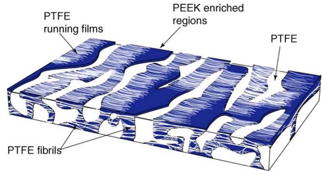
Fig. 3. An illustration of the targeted composite structure, where the major phase (PTFE) exists as neat regions interconnected via PTFE fibrils. The PEEK-enriched material encasing the neat regions of PTFE may also be interconnected. The PTFE running films thought to be responsible for lubrication are shown originating from neat PTFE as noted and illustrated.
