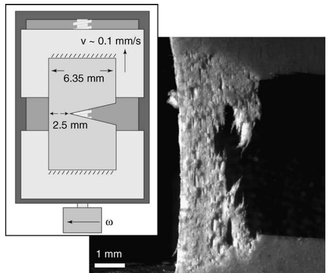
Fig. 12. Experimental schematic and resulting optical image of a notched fracture experiment for a 30 wt.% specimen under quasi-static extension at room temperature. The stress raiser does not induce a fracture response; instead, the material fibrillates in the direction of the stress and elongates an estimated 250–500% prior to breaking.
