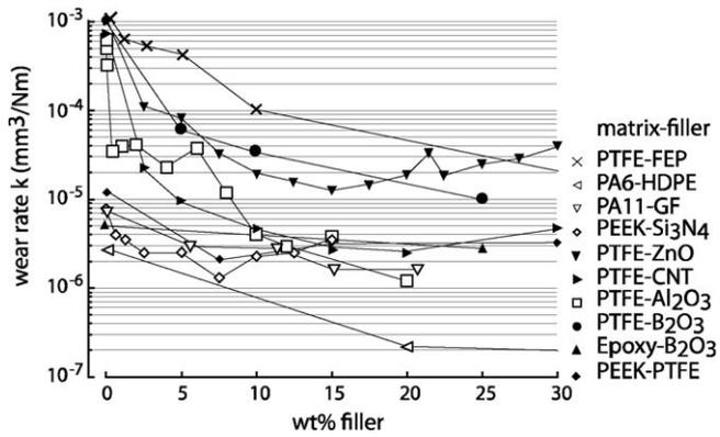
Fig. 1. Results from wear tests for representative polymer matrix composites found in the literature. Wear rate is plotted vs. filler wt.%. PTFE-FEP [16], PA6-HDPE [17], PA11-GF [18], PEEK-Si<sub>3</sub>N<sub>4</sub> [19], PTFE-ZnO [20], PTFE-CNT [21], PTFE-Al<sub>2</sub>O<sub>3</sub> [21], PTFE-B<sub>2</sub>O<sub>3</sub> [22], Epoxy-B<sub>2</sub>O<sub>3</sub> [22], and PEEK-PTFE [2].
