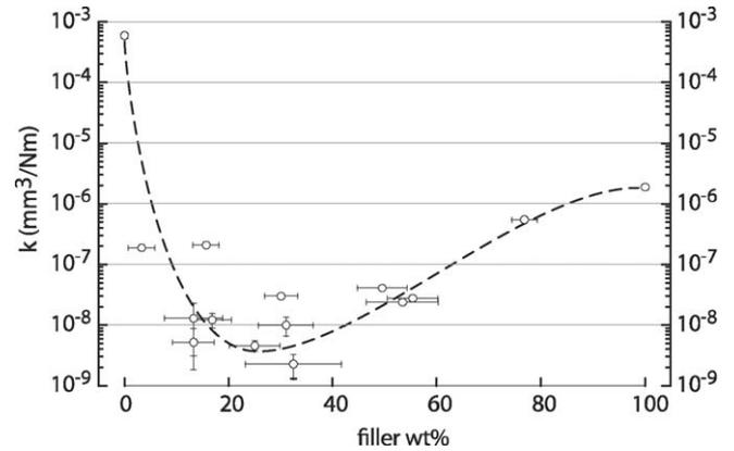
Fig. 7. Wear rates calculated from interrupted mass measurements for the composites plotted as a function of PEEK filler wt.% as calculated using the measured sample density. The uncertainty intervals on wear rate are calculated according to [13], while the horizontal confidence intervals are calculated following Eqs. (1) and (2). Sample surfaces are 6.35 mm × 6.35 mm under 250 N of normal load and reciprocation length is 25.4 mm at a speed of 50.8 mm/s (the total sliding distance varied).
