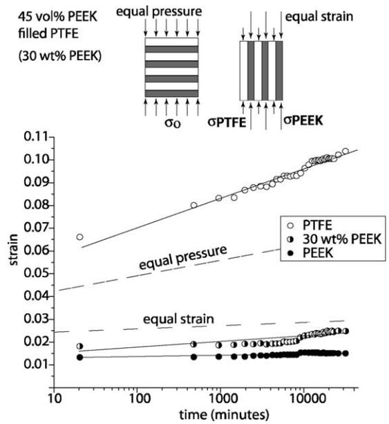
Fig. 11. Results of uniaxial compression tests of neat PEEK and PTFE as controls, and a 30 wt.% (45 vol.%) PEEK/PTFE composite. The responses of equal strain and equal pressure 45 vol.% composites were calculated based on the measured neat material responses, and are plotted with the data for comparison.
