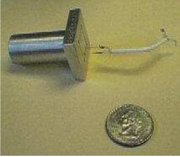
Fig. 2. A closer view of the scintillator mounted on the mobile robot.
