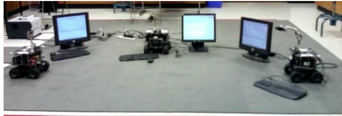
Fig. 7. The experimental set-up, where a CNN is implemented over a wireless network of three mobile robots.
