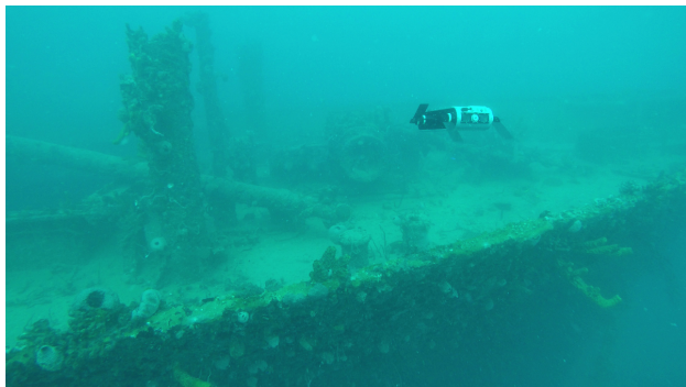
Fig. 1: Autonomous Underwater Vehicle over the Stavronikita shipwreck, Barbados.
