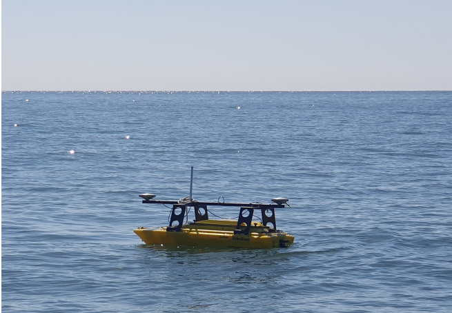
Fig. 6: The Echoboat 160 ASV, by Seafloor Systems Inc, can serve as an autonomous sensor platform for environmental surveys.
