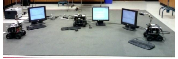
Fig. 4. A three-robot group used in the formation control experiments. The robots localize themselves using a motion capture system. Since their motion is subject to nonholonomic constraints, the control law is implemented by projecting the negated gradient direction on their feasible direction of motion.
