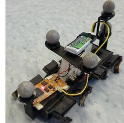
Fig. 1. The miniature eight-legged OctoRoACH robot [6].
