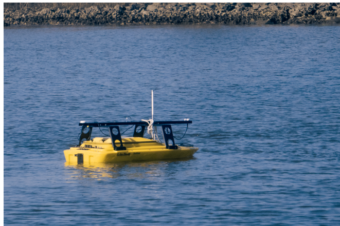
Fig. 1: Seafloor Systems Inc Echoboat 160 ASV can undertake missions such as environmental surveys, port security, and search and rescue operations.
