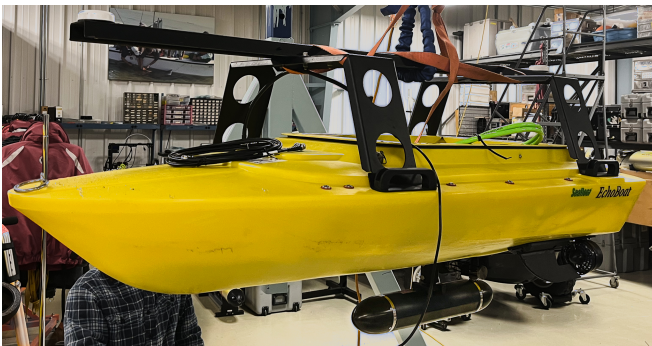
Fig. 5: Sensor setup for the UD Seafloor Systems Echoboat 160 ASV comprised of the Ping DSP 3DSS-DX interferometric sonar and SBG Ellipse-D3 dual GNSS antenna INS.
