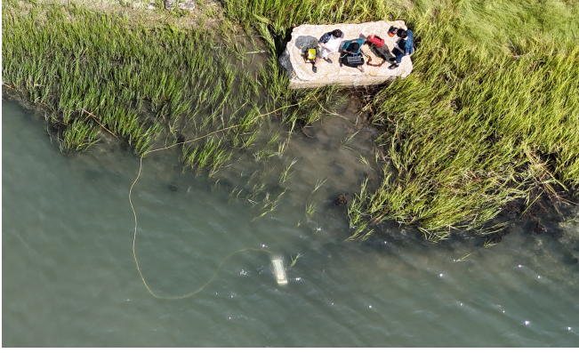
Fig. 3: Experimental deployment of the system, surveying a wild near-shore oyster reef in Lewes, DE. Operators can be seen teleoperating the Aqua2 and analyzing the feedback.
