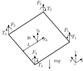
Fig. 3. A quadrotor helicopter configuration with roll(rotation along  $x$ -axis), pitch(rotation along  $y$ -axis), yaw(rotation along  $z$ -axis), where the Euler angles are  $\psi, \theta$ , and  $\phi$  respectively.
