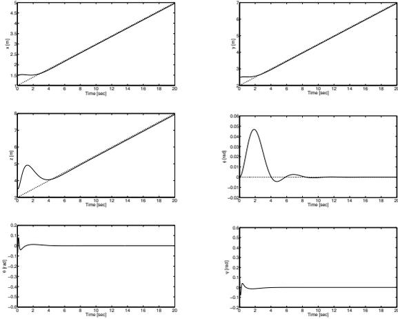
Fig. 5. Position and attitude of the quadrotor using the three-level hierarchical controller. The dash lines are the desired trajectories for flat outputs  $y_d = \eta_d = z$ .
