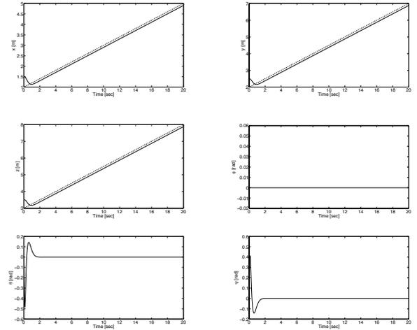
Fig. 4. Quadrotor position and attitude using the two-level hierarchical controller. The dash lines are the desired trajectories for flat outputs  $y_d = \eta_d = z$ .
