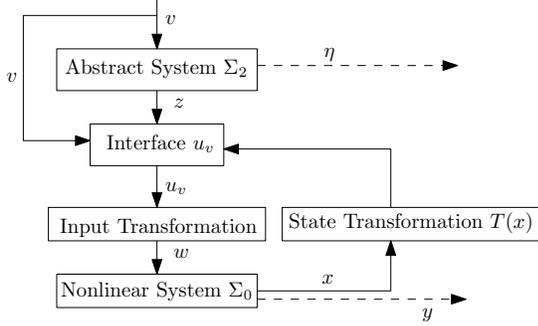
Fig. 1. A two-level hierarchical control system architecture. The scheme enables planning and control using models of smaller dimension when the concrete nonlinear model  $\Sigma_0$  is differentially flat.
