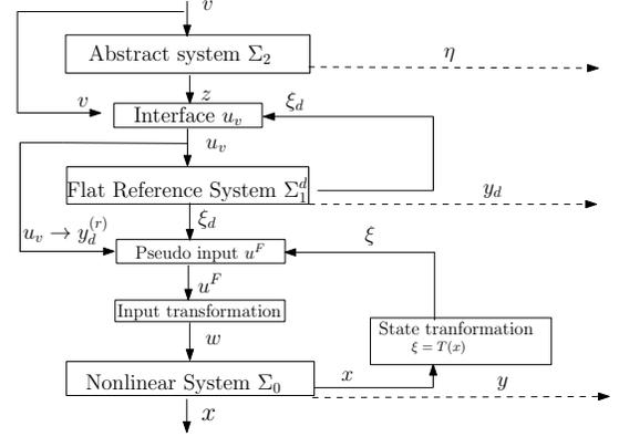
Fig. 2. A three-level hierarchical control system architecture. It applies to nonlinear systems that can be made differentially flat after some approximations. An additional control loop is established through  $u^F$  to mitigate the effect of the approximation.
