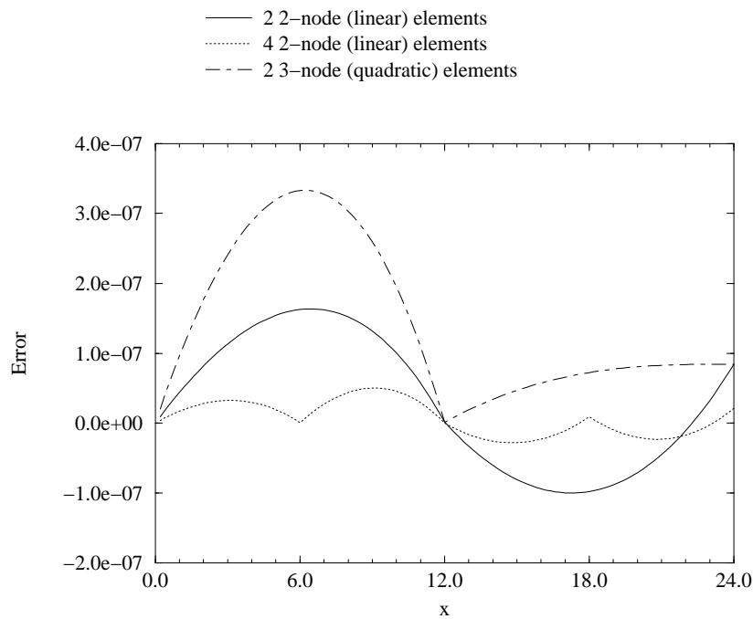
Note that the solution is less accurate if quadratic elements are used. This could be due to the fact that the exact solution is mostly linear than quadratic.
