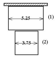
$$\begin{split} -\int_{0}^{24} AE \frac{dq}{dx} \frac{d\phi}{dx} dx &= -\int_{0}^{12} A^{(1)} E \frac{q_{1} - q_{0}}{12} \frac{\phi_{1} - \phi_{0}}{12} dx - \int_{12}^{24} A^{(2)} E \frac{q_{2} - q_{1}}{12} \frac{\phi_{2} - \phi_{1}}{12} dx \\ &= -(\phi_{1}, \phi_{2}) \begin{bmatrix} \frac{5.25 + 3.75}{12} & -\frac{3.75}{12} \\ -\frac{3.75}{12} & \frac{3.75}{12} \end{bmatrix} \begin{bmatrix} q_{1} \\ q_{2} \end{bmatrix} E \end{split}$$
