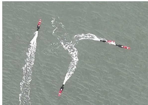
Fig. 1: A small fleet of four Jaiabots as they reconfigure themselves to achieve a group control objective.
