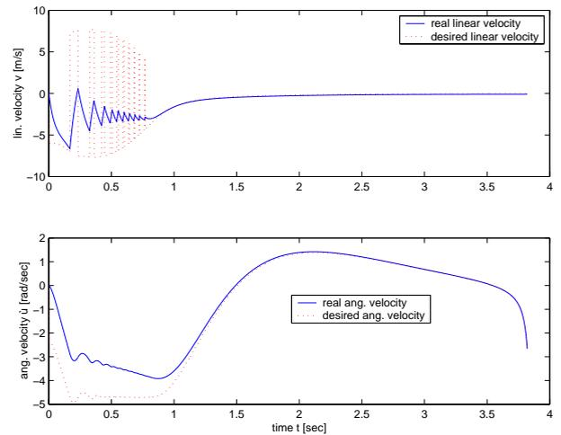
Figure 5: Filtering of chattering through backstepping
