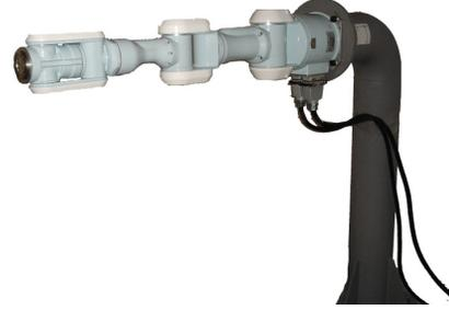
Fig. 3. Mitsubishi PA10-7C robotic manipulator configuration, with 7 d.o.f.
