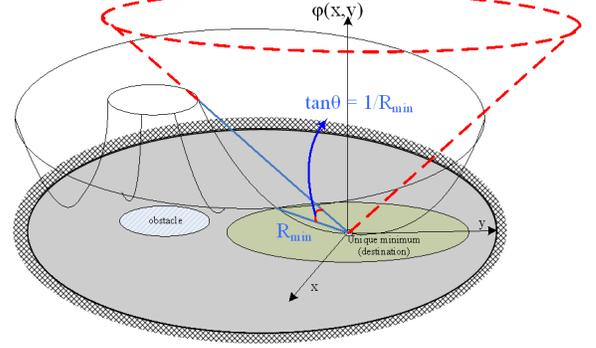
Fig. 6. A navigation function over a free configuration space.
