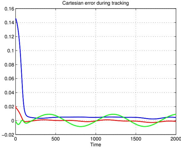
Fig. 12. *Scenario Simulation Results*: Cartesian position error between the real position of the robot and the predefined trajectory during trajectory tracking, blue -  $x$ , red -  $y$ , green -  $z$ .
